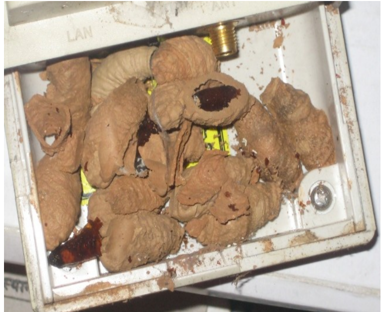
Fig: Haat Engenius Radio made faulty by Insect insect
